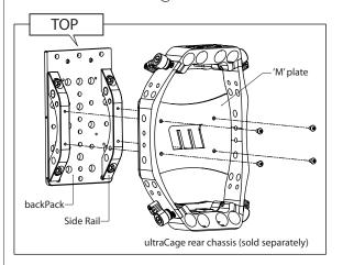
Align backPack with ultraCage as shown, making sure the top side is facing up. From inside the cage, tighten 4 provided screws from the 'M' Plate into the side rails of the backPack.
